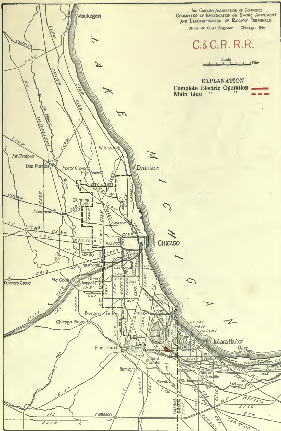
FIG. 549. TRACKAGE TO BE ELECTRIFIED BY THE CHICAGO & CALUMET RIVER RAILROAD
